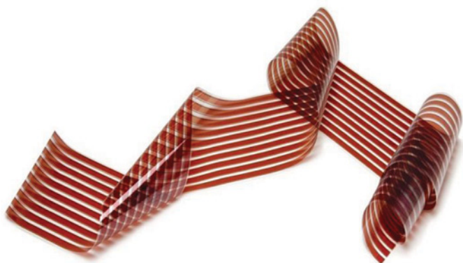
Fig. 1. Organic cells are flexible enough to be bent and/or rolled. Image reproduced from Brabec and Durrant (2008) with kind permission from Cambridge University Press. (Figure available in color online.)
